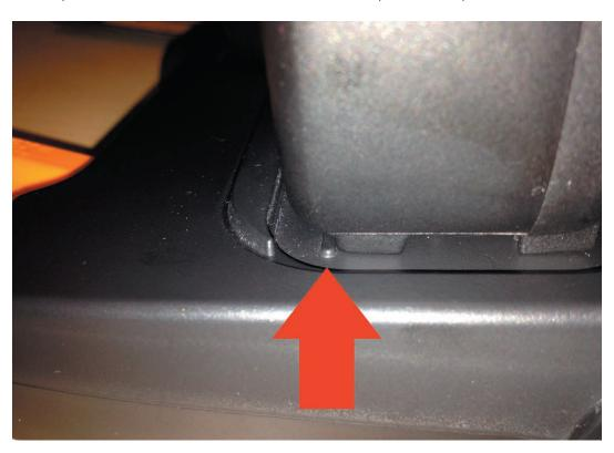
**NOTE.** Please ensure that the camera is fully engaged on the docking station – check that the front left camera foot is resting behind the protruding tab on the docking station (see image). The orange rubber battery cover should be rotated (do not bend!) and rested in the docking station recess – as this can affect connectivity between the camera and docking station
